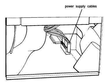
9. Lift the entire subassembly out of the computer and carefully place it on your work surface.
